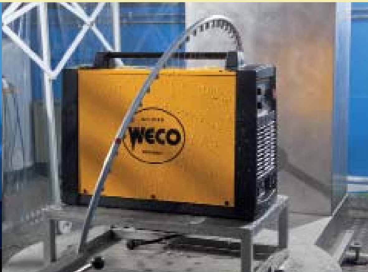
IP TEST: water proof test of the casing
